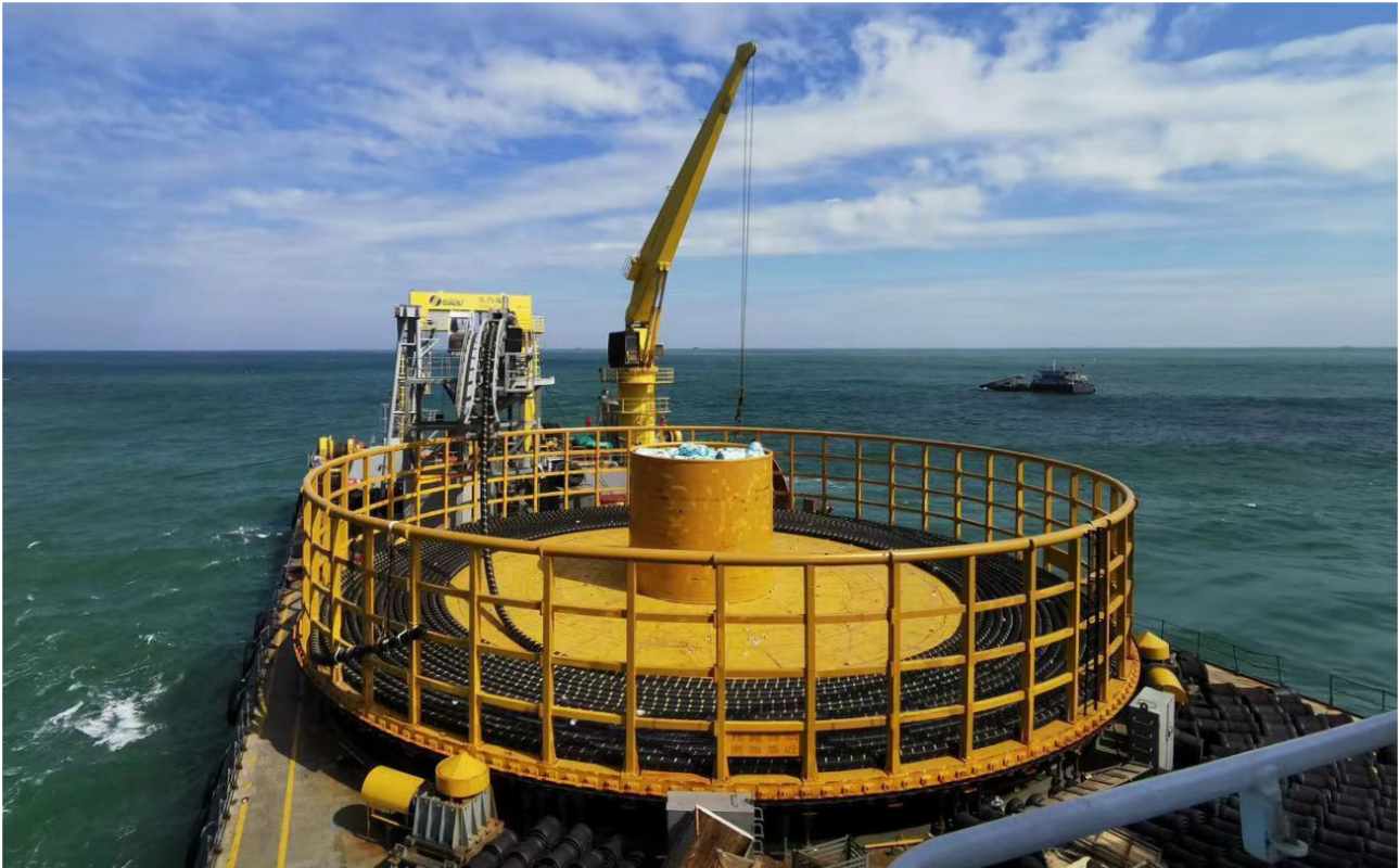
Submarine cables for power transmission to oil fields in Bohai Bay. (Photo courtesy of Ningbo Orient)
